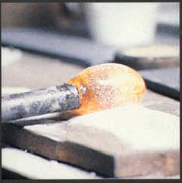
A gather of glass is taken on the pontil and rolled in sand
