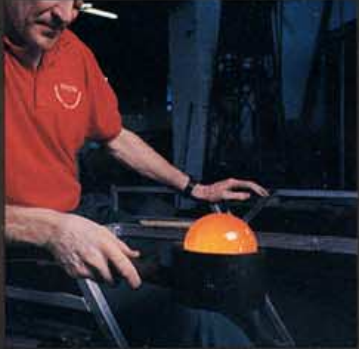
The spherical shape is carefully formed in a wooden block
