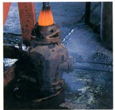
3. After carefully-controlled blowing in a wooden or metal mould, the vase can be cracked off onto a punty ready for the shaping of the neck.
