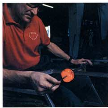
The glassmaker pushes holes into the soft glass to create air pockets
