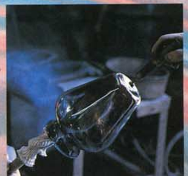
7. The Hartley Wood stamp of authenticity is applied to the base of the vase. The finished product is unmistakably Hartley Wood – English antique glass at its finest.
