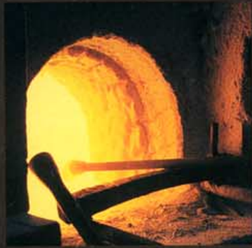
1. The first gather of molten glass is taken on the blowpipe.
