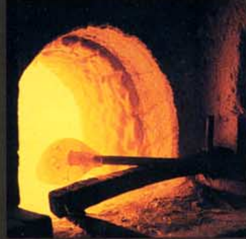
The third and final gather is taken, encapsulating the sand pattern and forming the air bubbles
