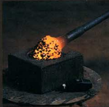
2. The gather is dipped in fragments of coloured glass which is melted and twisted, ready for a second gathering.
